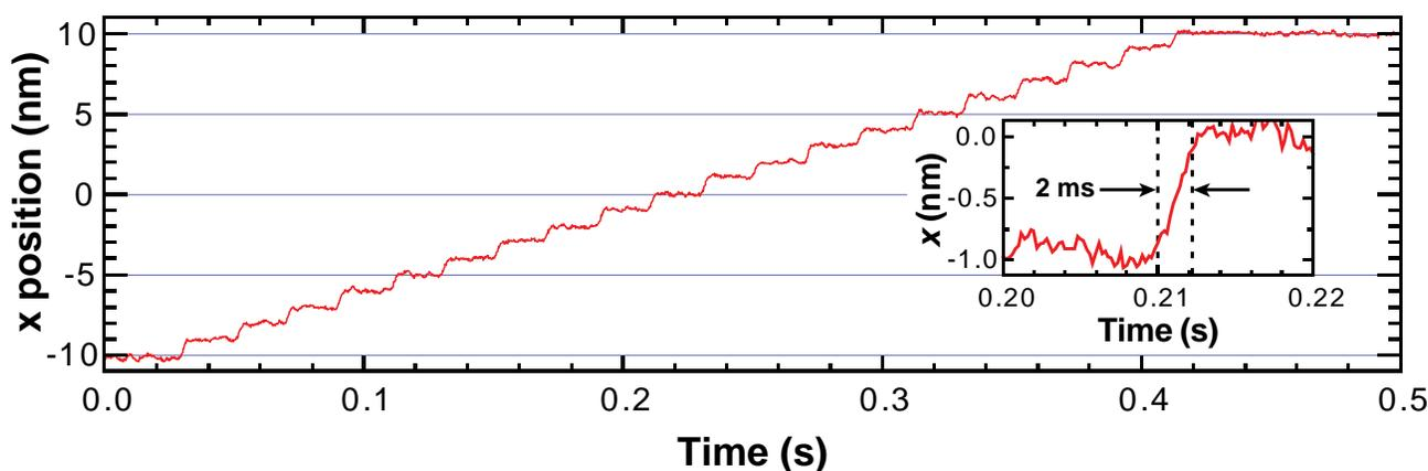
Fig. 4. Fast stepping enabled by parallel FPGA feedback control. (a) A record of sample position from a series of 1-nm steps filtered to 2 kHz. Sample position, independent of the servo-loop, was measured with the 845-nm laser. (Inset) Rise time for requested motion was  $\sim 2$  ms with the total step completed  $\sim 3$  ms after the request.
